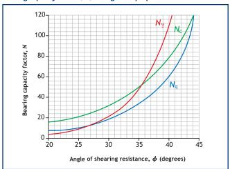
are needed. The formulation for the drained bearing capacity given in Figure 10 and Panel 4 assumes that the groundwater level is at the underside of the base of the retaining wall. This will be conservative for situations where groundwater can be guaranteed to be a distance  $\geq B$  below the wall base. Note that the overburden pressure used in the expression for bearing capacity is that due to backfill above the wall's toe (and is likely to be a small value).
