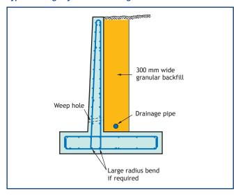
For walls with a high axial load (eg basement walls), the main reinforcement placed nearest to the wall faces should have transverse reinforcement in the form of links with at least four per  $m^2$  of wall area. Where welded mesh and bars of diameter  $\phi \leq 16$  mm are used with cover larger than  $2\phi$ , transverse reinforcement is not required.
