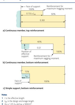
The shortest span must be greater than or equal to 0.85 times the longest span.
