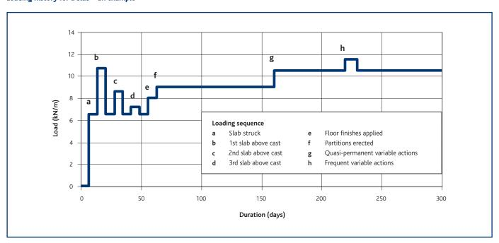
any of the earlier load stages. If, however, an earlier stage proves critical, the  $\xi$  value at that stage should be carried forward to all subsequent stages.
