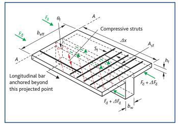
the interface of the flange and web can be resisted by the transverse reinforcement in the flange. The position of the neutral axis should be determined, and then the area of reinforcement can be calculated depending whether it lies in the flange or web (see Figure 11).
