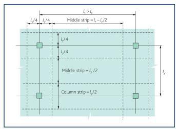
At internal columns, unless rigorous serviceability calculations are carried out, top reinforcement of area 0.5  $A_{\rm t}$  should be placed in a width equal to the sum of 0.125 times the panel width on either side of the column.  $A_{\rm t}$  represents the area of reinforcement required to resist the full negative moment from the sum of the two half panels each side of the column. It is also advisable to apply this requirement to perimeter columns as far as is possible.
