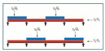
Figure 2 Adjacent spans loaded
