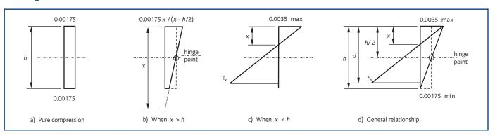
The general relationship is shown in Figure 8d). For concrete classes above C50/60 the principles are the same but the maximum strain values vary.
