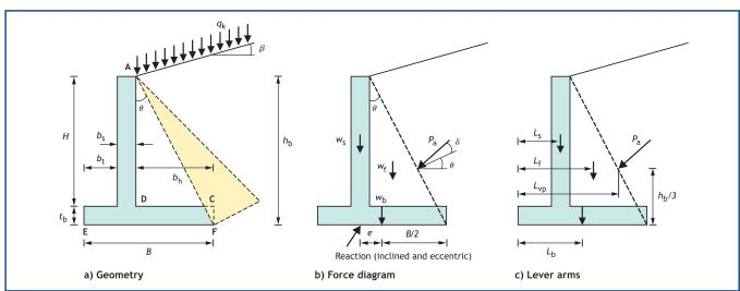
pressures acting on the **inclined** 'virtual' plane, AF. The earth thrust  $P_a$  (Figure 3b) is inclined at an angle  $\theta + \delta$  to the horizontal. (The same model is used to analyse plain concrete gravity walls.) The ground beneath the wall base must also be strong enough to carry the wall's self-weight and the downwards component of the earth thrust on the virtual plane.
